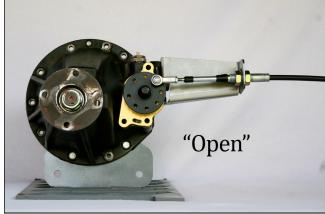
The cable should never bind or buckle when being cycled via the **Hand Shifter.** The key to this adjustment is to get the cable linkage to come close to the center of the lever without making contact.
